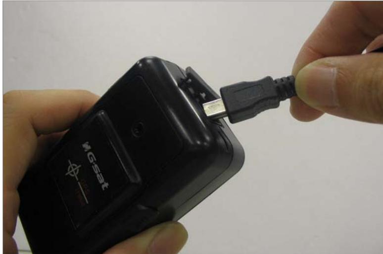
1. Fully charge the battery. Before your first time using of TR-150, please connect it with AC power adapter for battery charging under the power-off condition. (The included battery is specially designed for TR-150. Please do not use other type of battery; otherwise it will damage the device. If you need to change the battery for TR-150, please contact you local dealer.)
