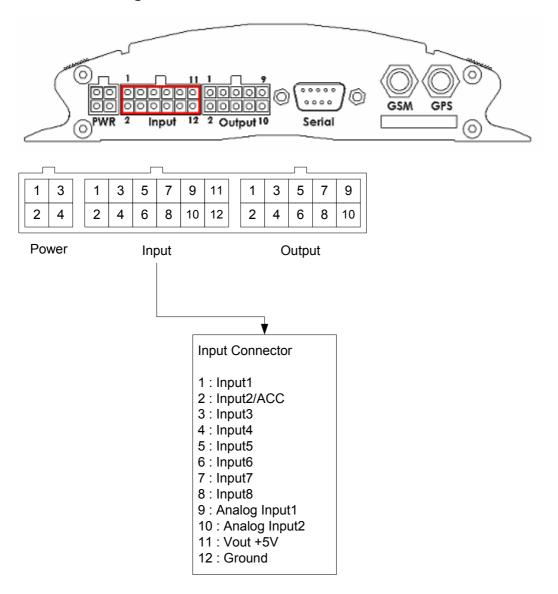
The Input number 1, 2 are positive triggered inputs and Input number 3, 4, 5, 6, 7, 8 are negative triggered inputs. If you would like to use power saving function, please connect the Input2/ACC to ACC wire. The analog inputs are reserved.
