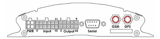
Connect GPS antenna to the GPS connector. The optimum location for the GPS antenna is on the roof of the vehicle. The covert and GPS antenna are directional, make sure they are facing up and laying as flat as possible. Secure them in place with glue, or zip ties.
